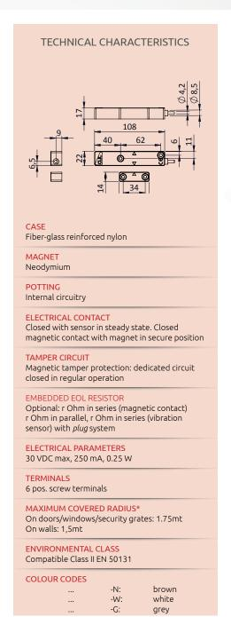
(\*) This is the maximum coverage when using VAS-series analysis boards. Coverage might decrease with other boards. Coverage might also be significantly affected by the door/window manterial, its type (fixed/openable), and the way it is fixed to walls. The same reasoning applies to the sensor's coverage area when mounted on walls.
